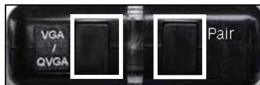
Figure 1.0 Press and hold the VGA/QVGA and Pair buttons at the same time
